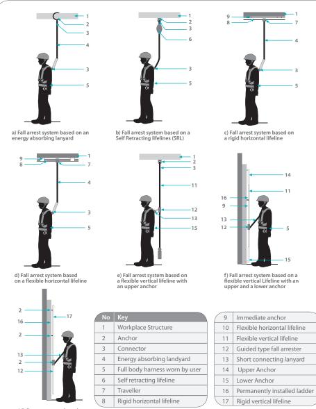
g) Fall arrest system based on a rigid vertical lifeline
