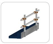
Figure 30: Example of edge protection off the structure.
