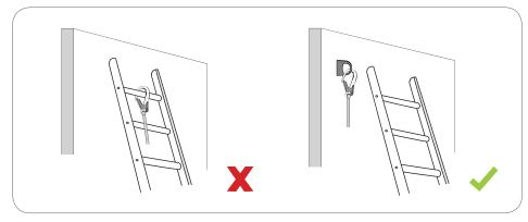
Figure 8: Fall prevention systems should not be connected directly to portable ladders that are leaned against any structures for the purpose of access. It should be connected to a proper anchorage adjacent to the ladder. A connection to a portable ladder should only be made if the top of the ladder is properly secured and the system tested by a competent person.
