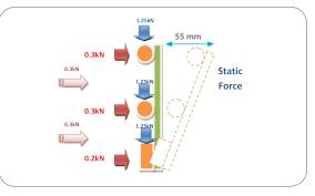
Figure 25: Static loading requirements for Class A system.
