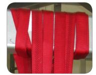
Figure 7: Excessive looping of an anchor sling should be avoided (unless otherwise stated in manufacturer's manual).
