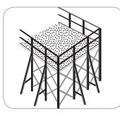
Figure 29: Example of ground supported edge protection.
