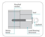
Figure 5: Example of chemically bonded anchor.
