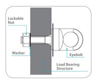
Figure 4: Example of a throughtype anchor.
