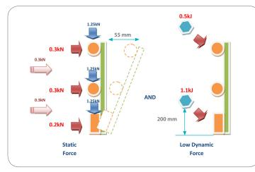
Figure 26: Loading requirements for Class B system.
