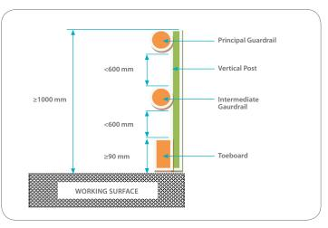
Figure 24: Dimension requirements for a temporary edge protection system.
