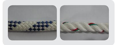
Figure 10: Examples showing a kernmantel (left) and hawser-laid lifeline.
