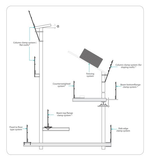
\* Adapted for use on roofs (as edge protection)
